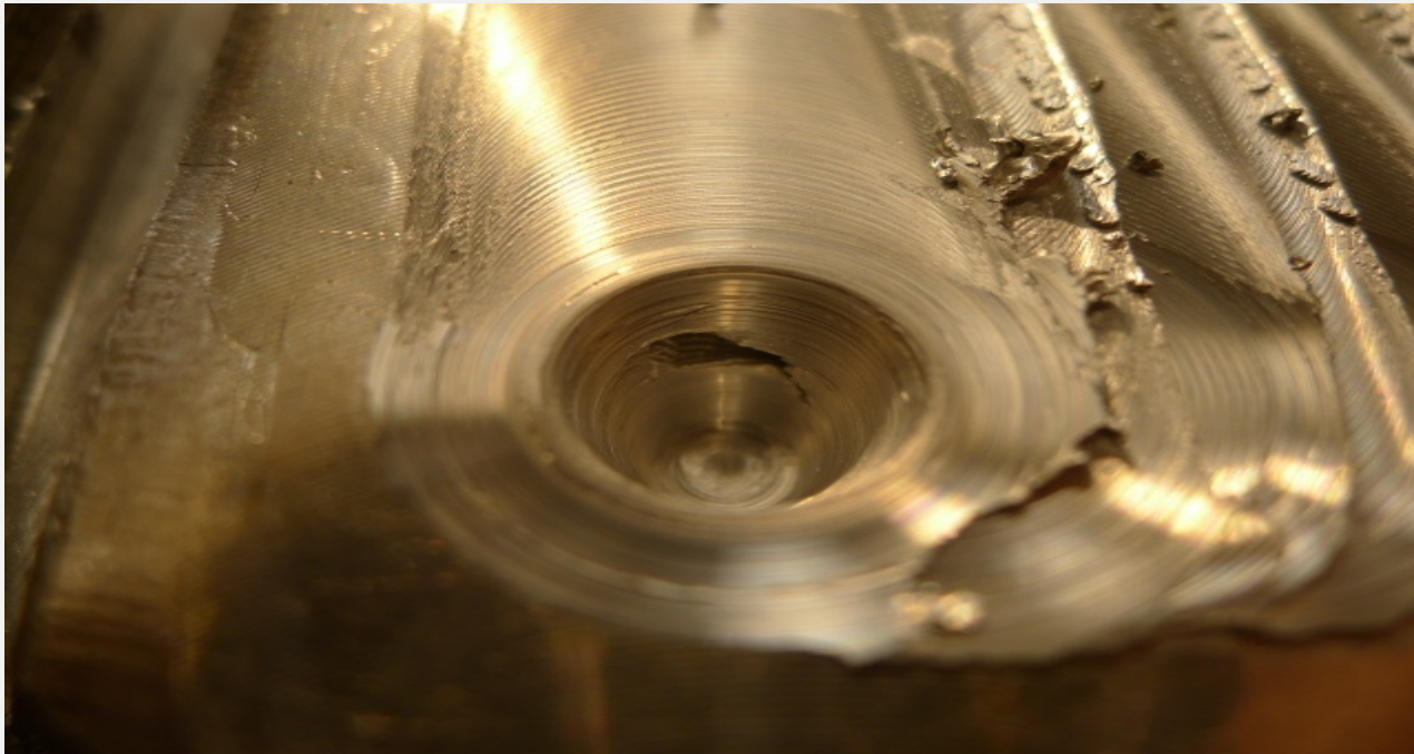
Longitudinal void in WJ made of pure Al 10 mm in thickness
